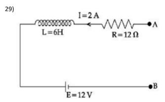
As per the given figure, if  $\frac{dI}{dt}$  = -1 A/s then the value of V<sub>AB</sub> at this instant will be \_\_\_\_\_\_V
